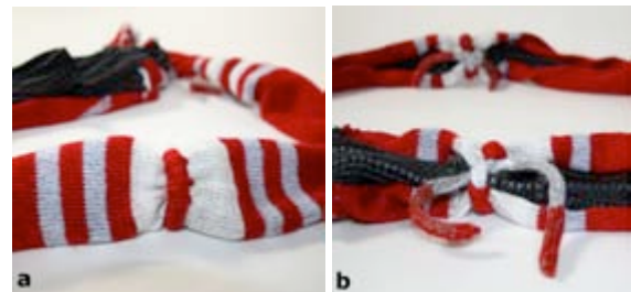
Figure 3. Active zones a) White areas act as the location switches. Grey lines are direction indicators. b) A closed string switch.
