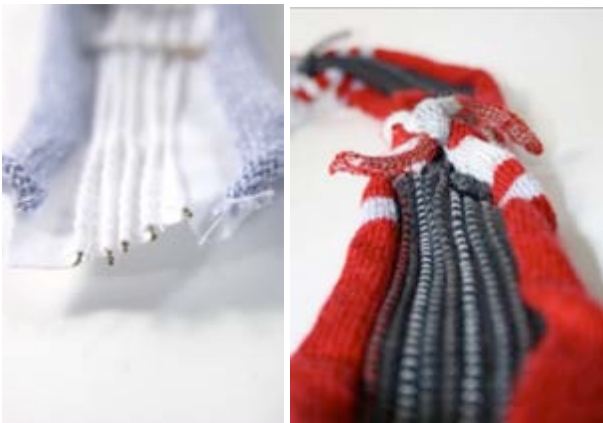
Figure 7. Close ups of the rows stitched in the jersey to carry the data lines securely.
