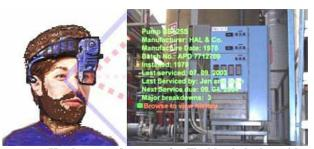
Figure 6: Head mounted concept for Flashback device, with its foldable visor, projecting the Log of the equipment's activities like hologram in the view of the worker; the projected image can also be pictures or video footages of past repair activities by the experienced for situated, peripheral learning at the scene of problem solving by the novice
