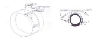
Figure 12 Sketches of the pulsemeter as either a bracelet or a ring.
