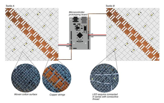
Figure 2: Digital textile prototype 1: Woven cotton surfaces with embedded copper wires and LEDs on the sides. Microcontroller prototyping board in the center.
