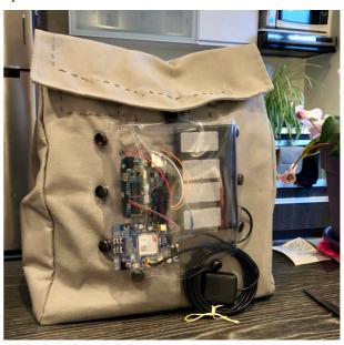
Figure 5: The final iteration of La Encomienda. In the front, the textile bag has a plastic pocket that contains a microcontroller prototyping board, a cellular module, an antenna and a packet of AA batteries.
